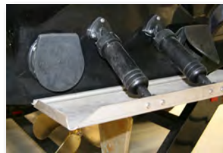
Ski boat ballast water lines.
